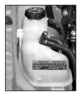
The coolant level should be at the FULL COLD mark. If it isn't, you may have a leak at the pressure cap or in the radiator hoses, heater hoses, radiator, water pump or somewhere in the cooling system. If there seems to be no leak, with the engine on, check to see if the electric engine cooling fan is running. If the engine is overheating, the fan should be running. If it isn't, your vehicle needs service.
