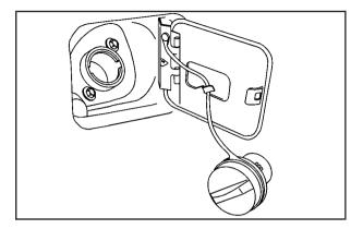
While refueling, hang the tethered fuel cap from the hook on the fuel door.
