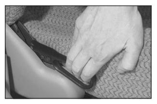
To adjust the seatback, lift the lever located on the outboard side of the seat and move the seatback to where you want it. Release the lever and push rearward on the seatback to make sure it is locked. Pull up on the lever without pushing on the seatback and the seatback will go to an upright position.
