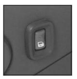
If your vehicle has this feature, you can lock or unlock all the doors on your vehicle from the driver's or front passenger's door lock switch.
