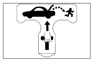
*Notice:* Using the emergency trunk release handle as a tie-down or anchor point when securing items in the trunk may damage it. Use the emergency trunk release handle only to help you open the trunk lid.
