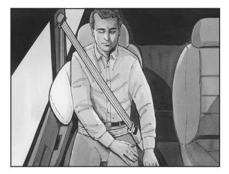
If your vehicle has one, the passenger's side impact air bag is in the side of the passenger's seatback closest to the door.
