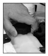
5. Then replace the pressure cap. Be sure the pressure cap is hand-tight and fully seated. See your dealer, if necessary.
