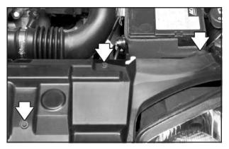
1. Remove the plastic fasteners from the shield. Use a tool to pry up the center of the fastener. Be careful not to break the fasteners that hold the shield in place.
