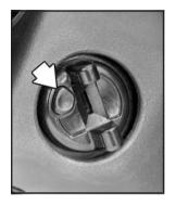
The ignition key cannot be removed from the ignition unless the key release button is used.
