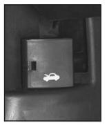
1. Pull the handle located inside the vehicle on the driver's side under the instrument panel.
