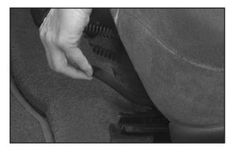
Lift the lever located on the front of the driver's seat to unlock it. Slide the seat to where you want it and release the lever. Then try to move the seat with your body, to make sure the seat is locked into place.
