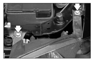
2. Remove the two bolts from the headlamp assembly. Pull the headlamp assembly up and toward the front of the vehicle to access the bulb assembly.
