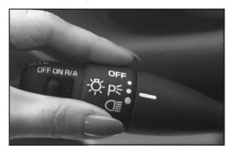
The exterior lamp band on the turn signal/multifunction lever controls the exterior lamps.
