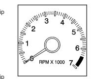
The tachometer displays the engine speed in revolutions per minute (rpm).
