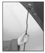
Lift the hood, release the hood prop from its retainer and put the hood prop into the slot in the hood marked by an arrow. Use the prop rod sleeve when handling the hood prop.
