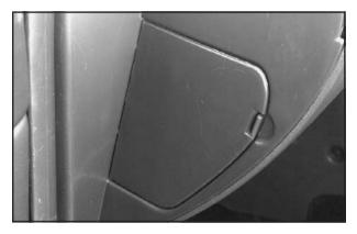
The instrument panel fuse block is located on the driver's side of the instrument panel. To open, push the tab on the access door to the left and pull the door forward. Make sure to insert the tabs when replacing the cover.
