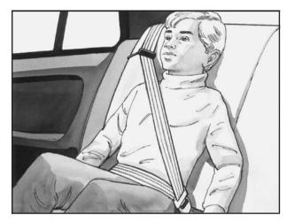
4. Buckle, position and release the safety belt as described in *Rear Seat Passengers on page 1-23.* Make sure that the shoulder belt crosses the shoulder.
