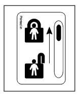
If your vehicle is a four-door model, it is equipped with rear door security locks that help prevent passengers from opening the rear doors on your vehicle from the inside.
