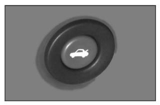
Press the remote trunk release button, located on the lower left side of the instrument panel, to release the trunk lid.
