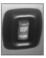
Your vehicle may have a sunroof. With the ignition on, press and hold the rear of the switch and the glass panel will open to the vent position.
