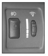
The button for your fog lamps is located next to the instrument panel brightness control.
