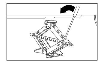
9. Lower the vehicle by turning the jack handle counterclockwise. Lower the jack completely.
