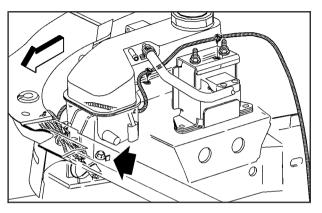
If your vehicle has this feature, in very cold weather 0°F (-18°C) or colder, the engine coolant heater can help. You'll get easier starting and better fuel economy during engine warm-up. Usually, the coolant heater should be plugged in a minimum of four hours prior to starting your vehicle. At temperatures above 32°F (0°C), use of the coolant heater is not required.
