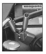
Don't let the other end touch metal. Connect it to the positive (+) terminal of the good battery. Use a remote positive (+) terminal if the vehicle has one. Don't let the other end touch anything until the next step. The other end of the negative (–) cable *doesn't* go to the dead battery. It goes to a heavy, unpainted metal part or to a remote negative (–) terminal on the vehicle with the dead battery.
