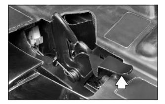
2. Then go to the front of the vehicle and lift up on the secondary hood release lever. The secondary hood release lever is located near the front center of the hood toward the driver's side.
