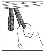
1. Pull the release straps located in the trunk. The right strap operates the passenger's side rear split seat. The left strap operates the driver's side rear split seat.
