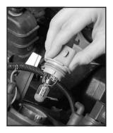
6. Remove the bulb by pulling it straight out.
