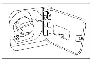
The tethered fuel cap is located behind a hinged fuel door on the passenger's side of the vehicle.
