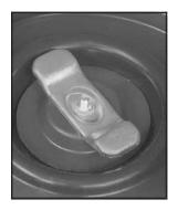
3. Turn the wing bolt counterclockwise and remove it. Then lift off the adapter and remove the compact spare tire.
