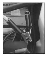
Now connect the black negative (-) cable to the negative (-) terminal of the good battery. Use a remote negative (-) terminal if the vehicle has one.
