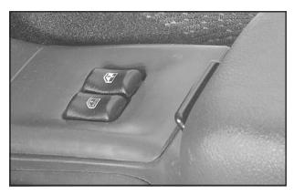
If your vehicle has this feature, the switches on the center console control each of the power windows when the ignition is on. In addition, on four-door models, each rear passenger door has a control switch for that window.
