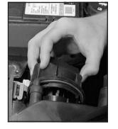
Remove the cover by turning it counterclockwise.
