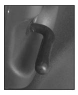
Adjust the driver's outside mirror with the control lever located on the driver's door.
